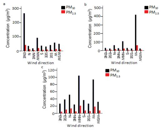
**Figure 4.** AWP values of ambient wind direction for the outdoor PM<sub>2.5</sub> and PM<sub>10</sub> concentrations in the operation room (a), pediatric (b), ICU (c) in Shahid Beheshti Hospital in 2015.
